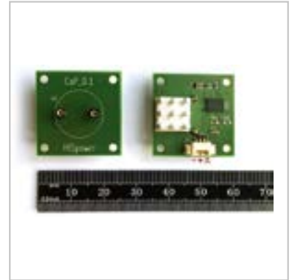
Driving circuit board for a quick evaluation of HISpower series IR emitters.
